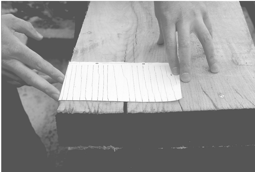
Fig. 10.4 Trace showing the rate of penetration of the bit under constant load, and showing the jump in alignment as the head passes through the split
