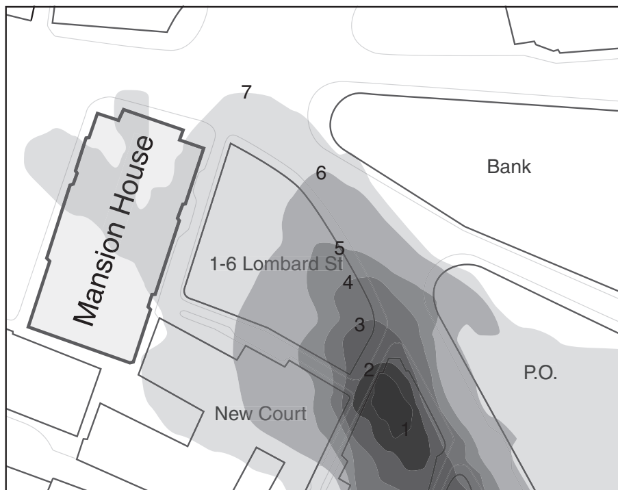
Figure 7.28 Developing settlement trough at the Mansion House, approaching.
