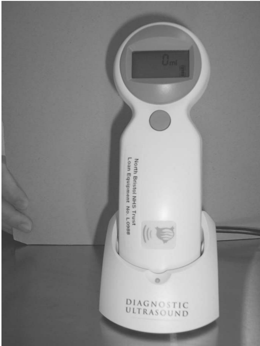
Fig. 3.24 Hand-held or patient-worn ultrasound machine which allows easy recording of bladder volume/post void residual, in clinic, on the ward or in the patient's home. The photo shows the ultrasound head, with display.
