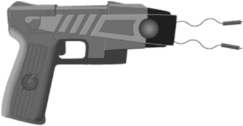
Fig. 2. Taser gun showing the device, its two probes, and the connecting wires.
