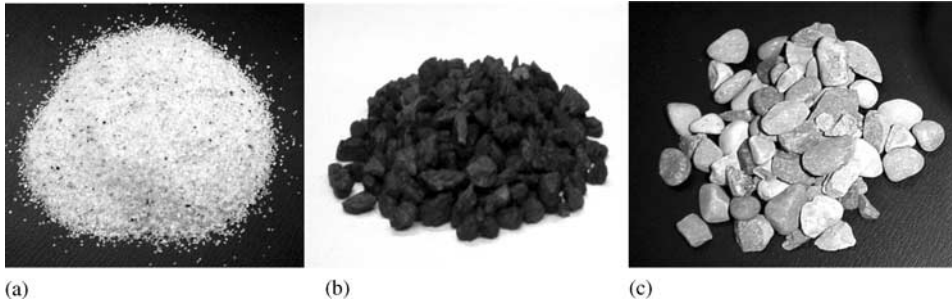
Figure 12. SAGEST TM filter materials (a) coarse sand; (b) activated carbon; (c) gravel. Each image is approximately 50 mm square.
