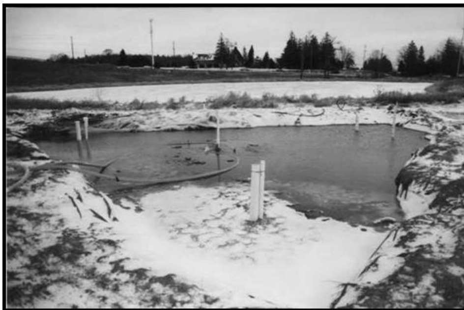
Figure 5. Field studies conducted during the winter months demonstrate that the filter blanket functions well in freezing conditions.
