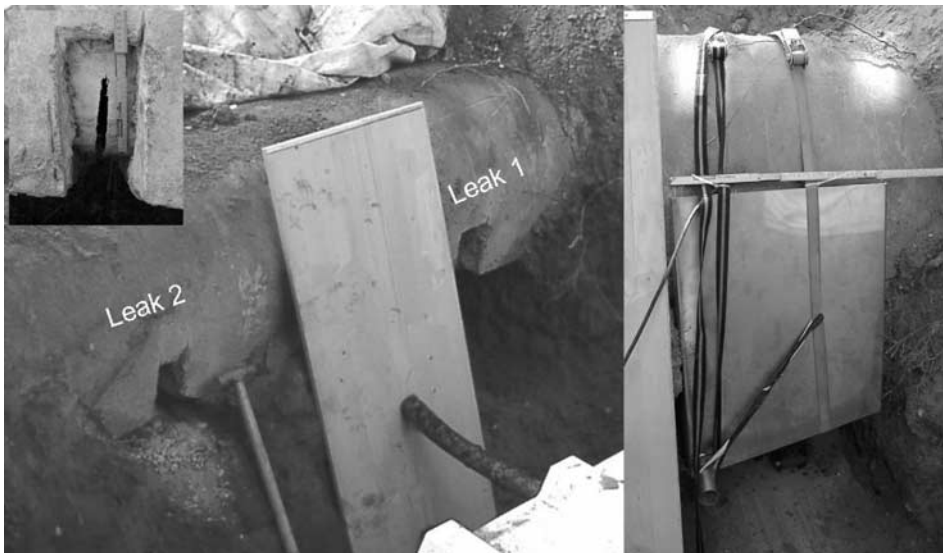
Figure 5. Excavated sewer during set-up of test site Kehler Strasse. Top left: detail of leak design, right: collecting tank underneath leak 1.
