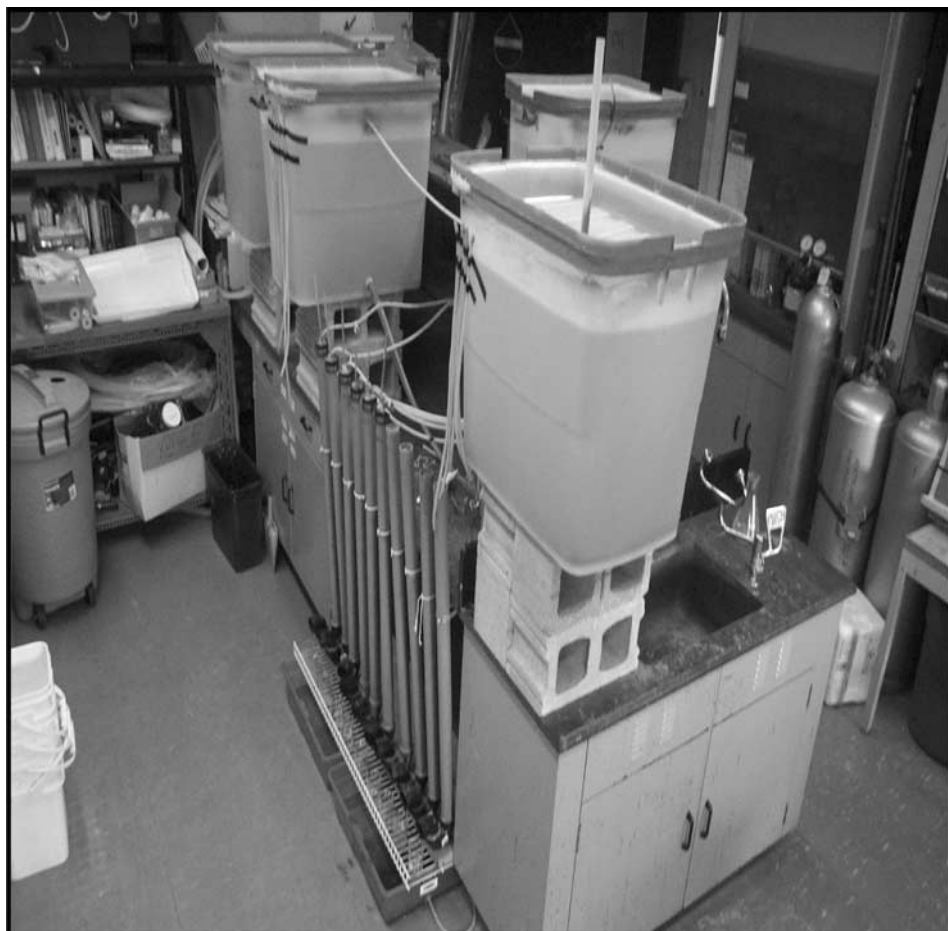
Figure 6. Experimental apparatus included a series of 10 drainage columns and a supply of both stormwater and distilled de-ionized water.
