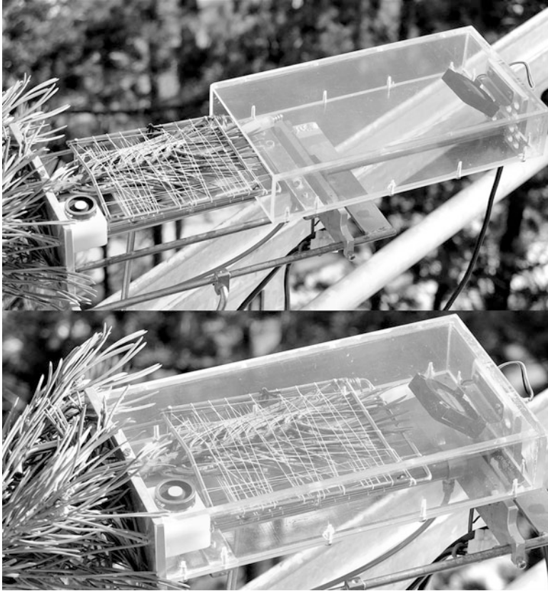
Fig. 9.7 An uncovered shoot experiences rain showers and full sunlight in a sliding measuring chamber. The chamber is open in the upper photo and closed in the lower photo. Photos: J. Aalto
