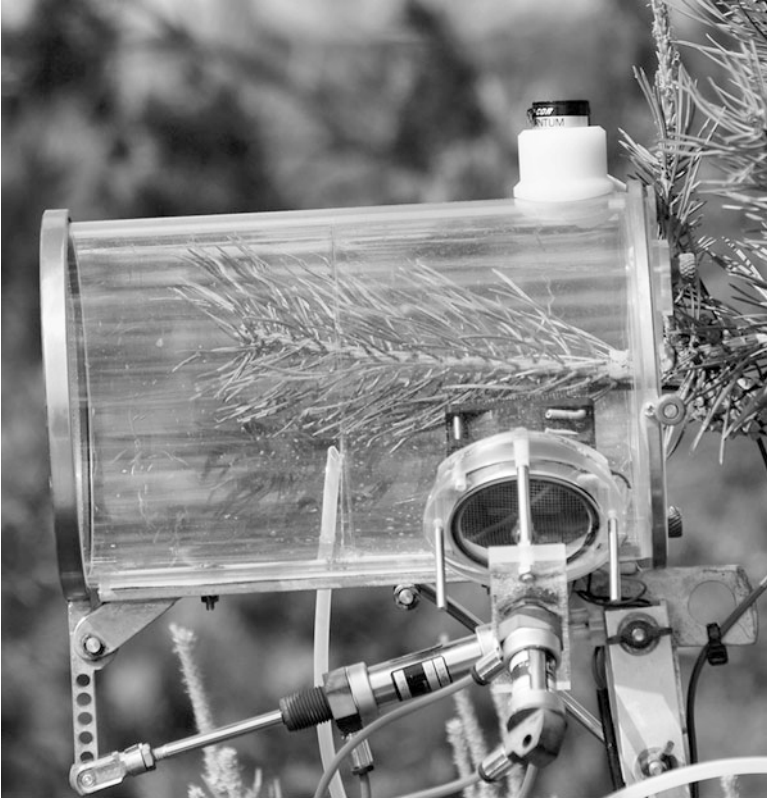
Fig. 9.6 The tube version of the measuring chamber when it is closed for measurements. Photo: J. Aalto
