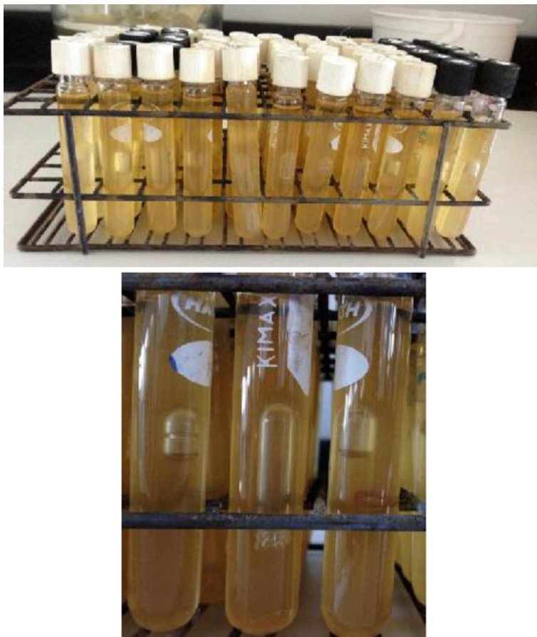
Fig. 3.5 Presumptive media inoculated with the disinfected water
