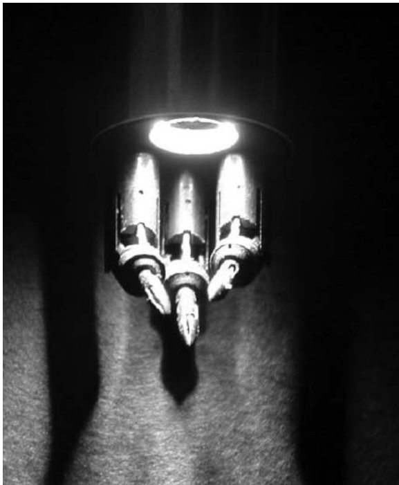
Fig. 3. Photograph of the tip of the slave manipulator. Three micro-forceps are installed, which are exchangeable during surgery
