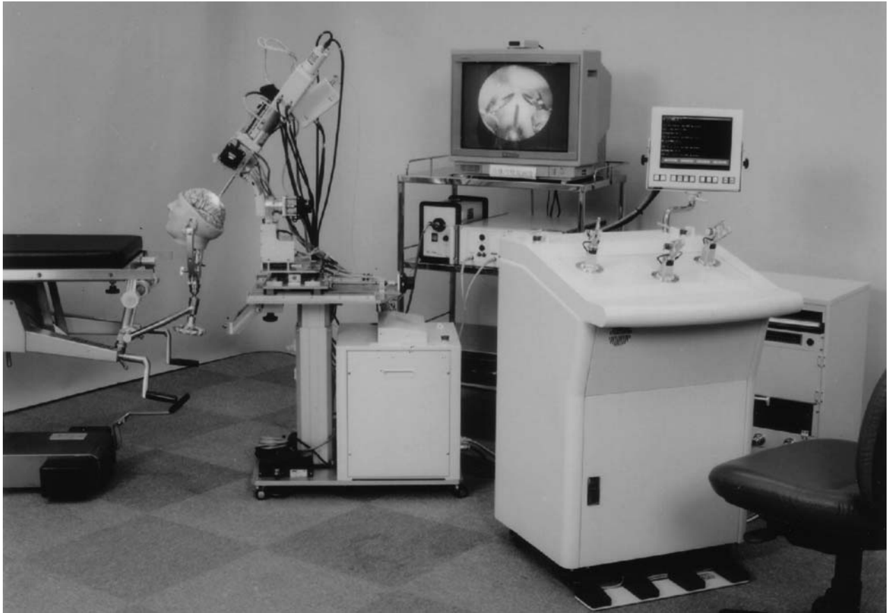
Fig. 1. Photograph of the NeuRobot system consisting of operating console, monitor and slave manipulator fixed in the supporting device
