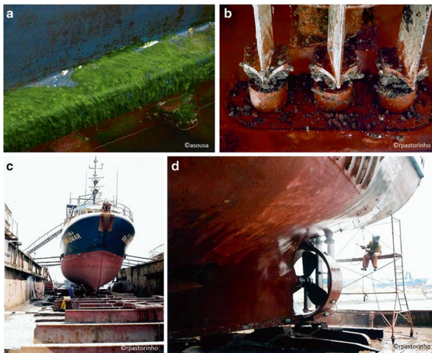
Fig. 4.2 Biofouling. When submerged into water, a community of algae and invertebrates develops in the ship's hull (a). Such community enhances corrosion in ships' essential structures (b) and increases roughness which in turn leads to an increase in hydrodynamic drag and fuel consumption. In order to overcome such problem the naval industry developed antifouling systems that prevent the attachment and growth of organisms in the submerged surfaces. The more effective the system, the larger periods a ship can spend at sea without need for dry-docking (c, d)
