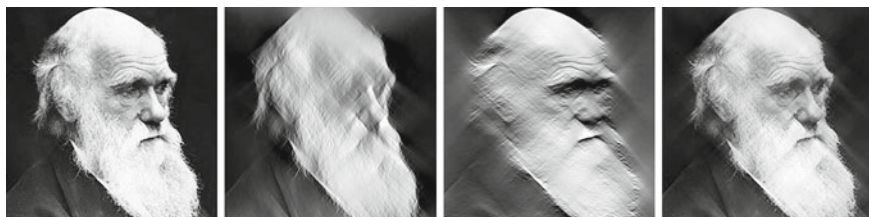
Fig. 1.15 Consequences of the missing wedge of tomography. From left to right : Original image; \pm 50^\circ tilt from the horizontal axis; \pm 50^\circ tilt from the vertical axis; averaging the two tomograms
