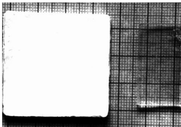
Fig. 6.14 Green compact of Aerosil OX before ( left ) and after sintering ( right )
