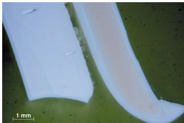
Fig. 8.31 Alumina deposit formed from alkaline aqueous suspension on zinc ( left ) and copper ( right ) electrode
