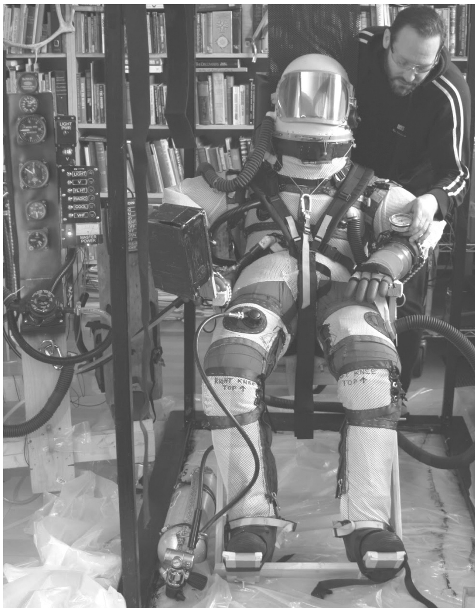
Figure 7.2. Home-Built Pressure Suit Developed by Cameron M. Smith. Photo by Cameron M. Smith.
