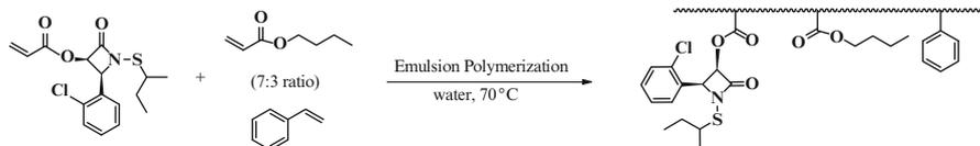
**Scheme 10** Preparation of  $\beta$ -lactam-conjugated polyacrylate nanoparticles by emulsion polymerization
