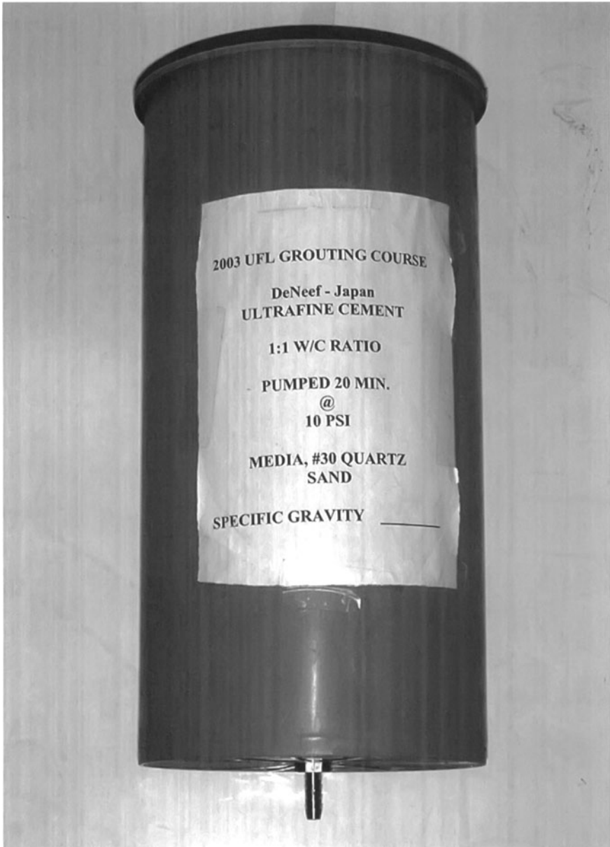
Figure 3-4. A concrete cylinder mold fitted with an injection valve.
