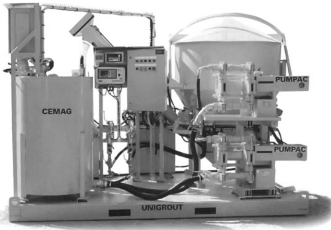
Figure 6-10. Atlas Copco grout plant with high-shear mixer.
