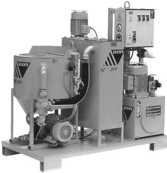
Figure 6-9. Hany grout plant with high-shear mixer.
