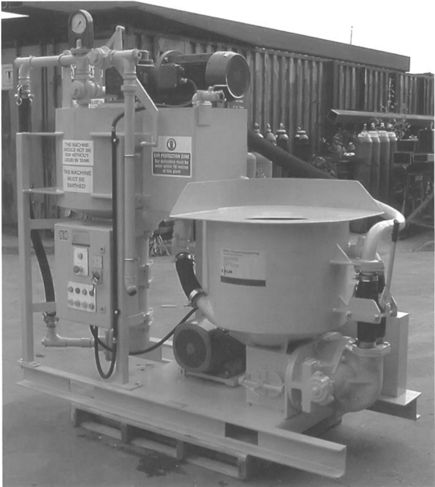
Figure 6-8. Colcrete grout plant with high-shear mixer.
