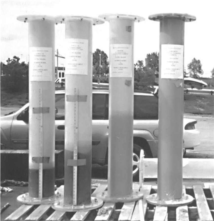
Figure 3-2. Grouts injected into sand columns. OPC grout is far left, OPC with superplasticizer is middle left, ultrafine cement-based grout is middle right, and ultrafine cement-based grout with superplasticizer is far right.
