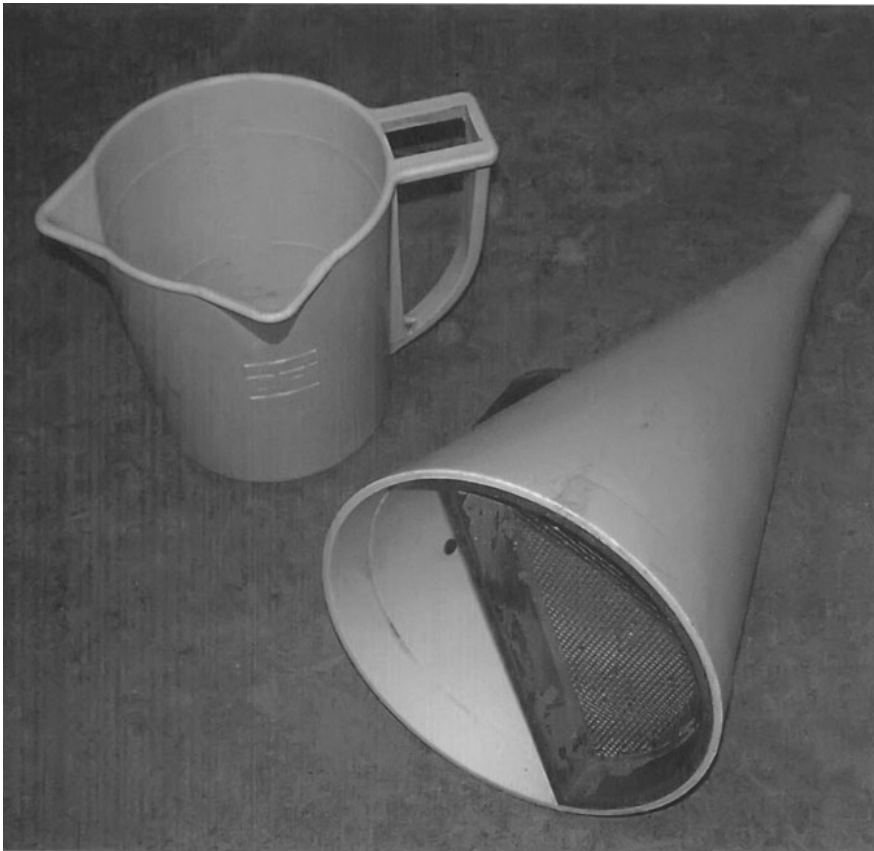
Figure 7-3. Marsh funnel and measurement cup.
