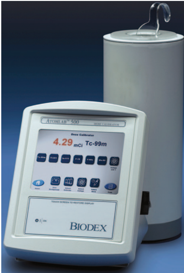
FIG. 7.5. A typical dose calibrator (Courtesy of Biodex Medical Systems, Inc, Shirley, NY).
