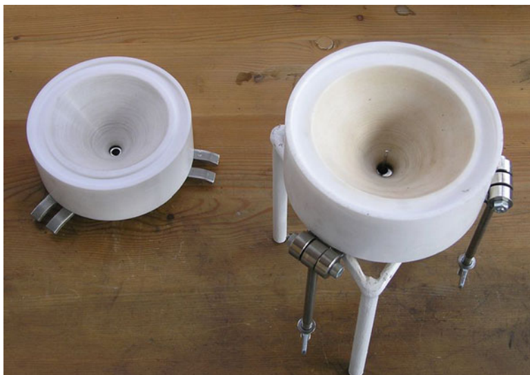
Fig. 13.8 Innovative 150 mm plane filter holder consisting of PTFE (Developed by TFZ)
