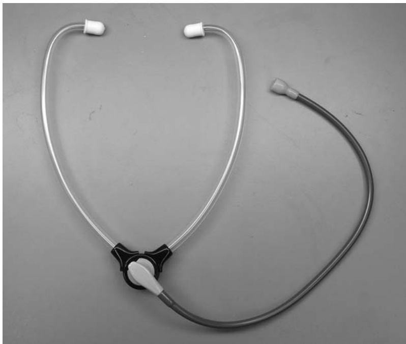
Figure 8.6 Illustration of a hearing instrument stethoscope used for a listening check.
