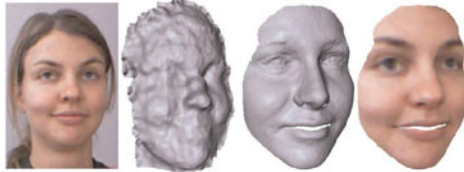
Figure 4.36 – Low-Cost Body Scanner: Avatar Enhancement adapted from Zollhöfer et al. [2011, p. 198]
