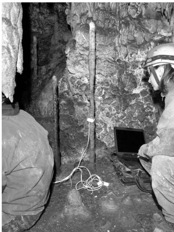
**Fig. 3.61** Dr. Katalin Gribovszki measuring the natural frequency of the stalagmite in Eminova Cave (photo G. Suranyi)
