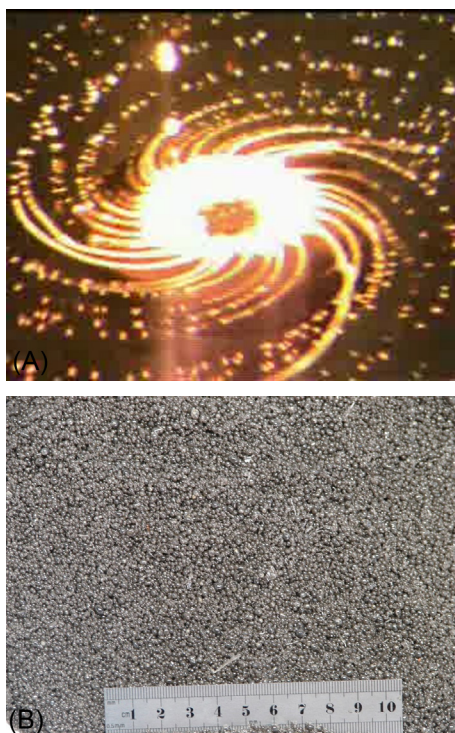
Fig. 5.8 (A) Still image of slag atomization on a spinning disc (1520°C and 1500 rpm) and (B) solid granules produced. Courtesy of Xie, Jahanshahi, and Norgate of CSIRO.
