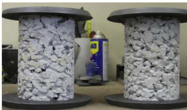
Fig. 11.16 Pervious concrete cylinders containing coarse EAF slag aggregate prior to compressive testing. It is competitive to normal aggregate concrete.
