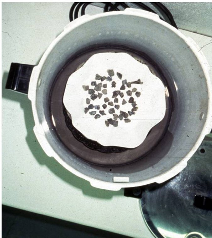
Fig. 12.10 View of slag particles following the autoclave disruption test.
