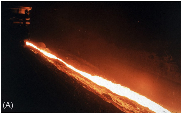
Fig. 8.4 The dumped molten ferronickel slag is fragmented by “thermal shock.” during ambient cooling in the slag storage area (A).
