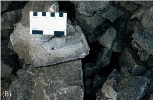
Fig. 8.4 Continued. Fragmented sized and crushed and screened to a wide range of gradations for highway construction uses (B).
