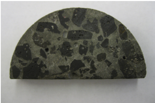
Fig. 12.11 Concrete containing steel slag coarse aggregate after autoclave testing.
