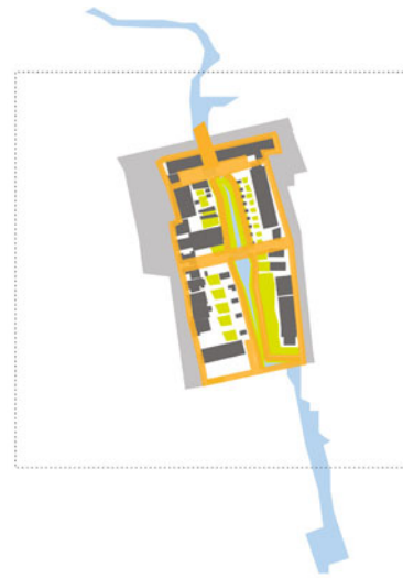
Figure 6.13a. Block plan A data for Bo01. Block area 10,004 m 2 ; 81 units; density 34 units/acre; building coverage 2,488 m 2 (25 percent); roads and parking 1,100 m 2 (11 percent); paths 1,443 m 2 (15 percent); green space 4,923 m 2 (49 percent). (Drawing by Nancy Nam; calculations by Harrison Fraker.)
