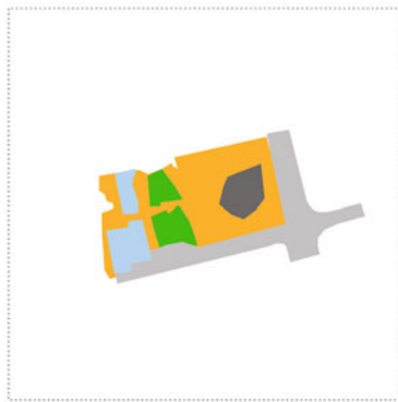
Figure 6.13b. Block plan B data for Bo01. Block area 3,600 m 2 ; 388 units; density 436 units/acre; building coverage 748 m 2 (20 percent); roads and parking 108 m 2 (3 percent); paths 2,027 m 2 (56 percent); green space 720 m 2 (20 percent). (Drawing by Nancy Nam; calculations by Harrison Fraker.)
