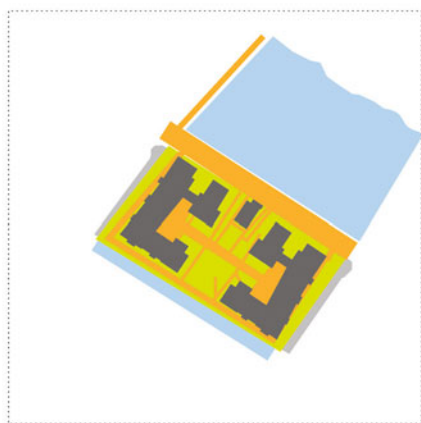
Figure 6.14b. Block plan B data for Hammarby Sjöstad. Block area 3,321 m 2 ; 101 units; density 123 units/acre; building coverage 2,031 m 2 (61 percent); roads and parking 66 m 2 (2 percent); paths 228 m 2 (6 percent); green space 1,062 m 2 (31 percent). (Drawing by Nancy Nam; calculations by Harrison Fraker.)
