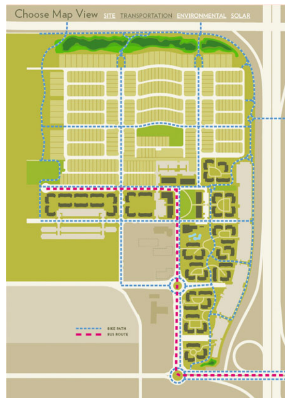
Figure 7.22. Bike and bus transit plan for West Village. (Source: West Village Community Partnership.)
