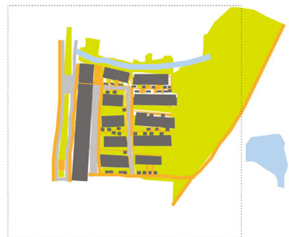
Figure 6.16c. Block plan C data for Vauban. Block area 10,226 m 2 ; 267 units; density 106 units/acre; building coverage 5,407 m 2 (52 percent); roads and parking 1,329 m 2 (13 percent); paths 532 m 2 (5 percent); green space 3,119 m 2 (30 percent). (Drawing by Nancy Nam; calculations by Harrison Fraker.)
