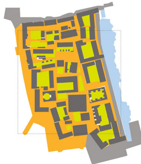
Figure 6.13c. Block plan C data for Bo01. Block area 48,995 m 2 ; 714 units; density 63 units/acre; building coverage 21,583 m 2 (44 percent); roads and parking 1,469 m 2 (3 percent); paths 17,398 m 2 (35 percent); green space 9,014 m 2 (18 percent). (Drawing by Nancy Nam; calculations by Harrison Fraker.)
