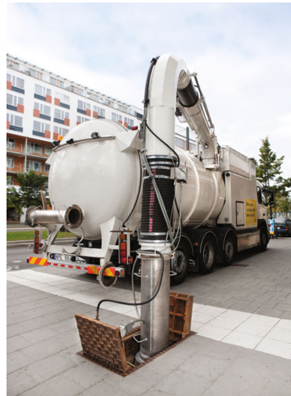
Figure 3.26. View of vacuum waste system collection in Hammarby Sjöstad. (Photograph by Lennart Johansson.)
