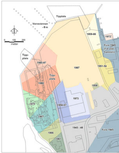
Figure 2.6. Plan showing dates and locations of different infill soils at Bo01. (Source: Formas [Swedish Research Council for Environment, Agricultural Sciences and Spatial Planning]; City of Malmö.)
