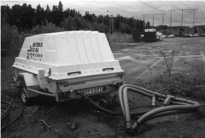
Figure 6.2 Mobile TRT device called “TED,” which was developed in Sweden. (Photo by Signhild Gehlin. From Gehlin, S., Thermal response test method development and evaluation. Ph.D. thesis, Department of Environmental Engineering, Lulea University of Technology, Lulea, 2002.)
