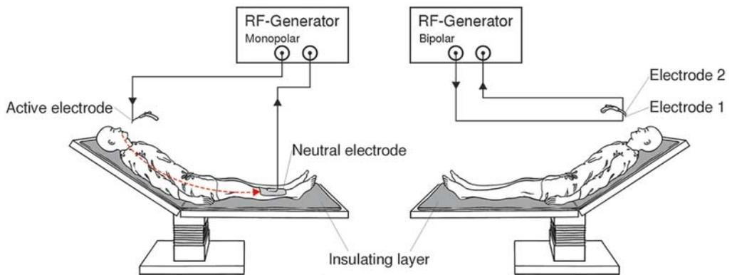
**Fig. 6.2.** Monopolar (i.e., Somnus) and bipolar (i.e., Celon) systems for interstitial radiofrequency surgery
