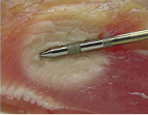
**Fig. 6.1.** Interstitial application of radiofrequency energy via needle electrode, shown here in turkey hen meat using the Celon system (RFITT, Celon, Teltow, Germany)
