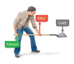
(b) Mechanical disadvantage with a speed lever
