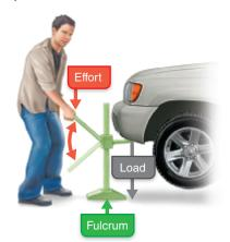
(a) Mechanical advantage with a power lever
