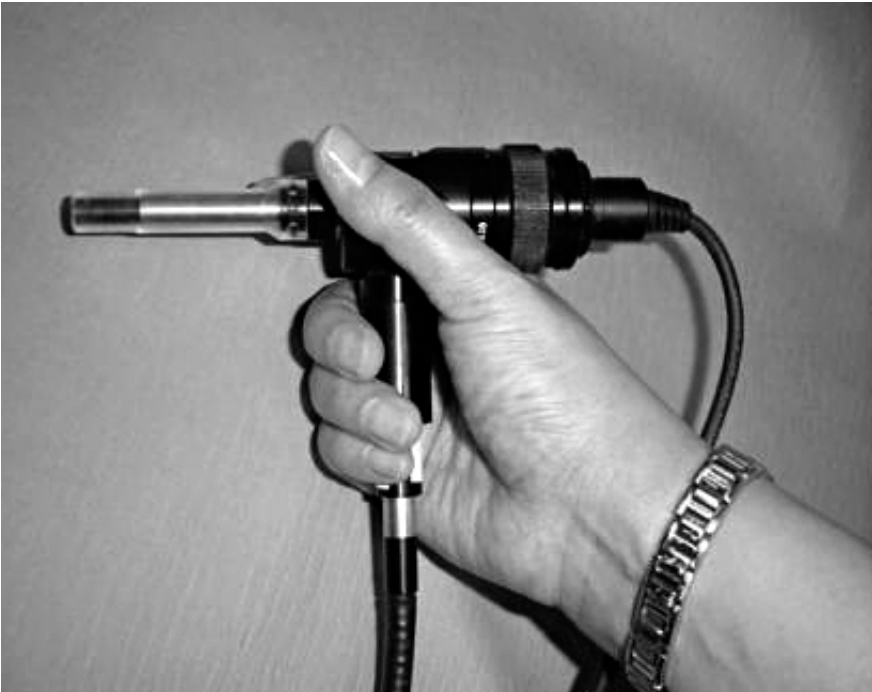
Fig. 2. Orthogonal polarisation spectral imaging camera: CYTOSCAN A/R (Cytometrics Inc., Philadelphia, PA)
