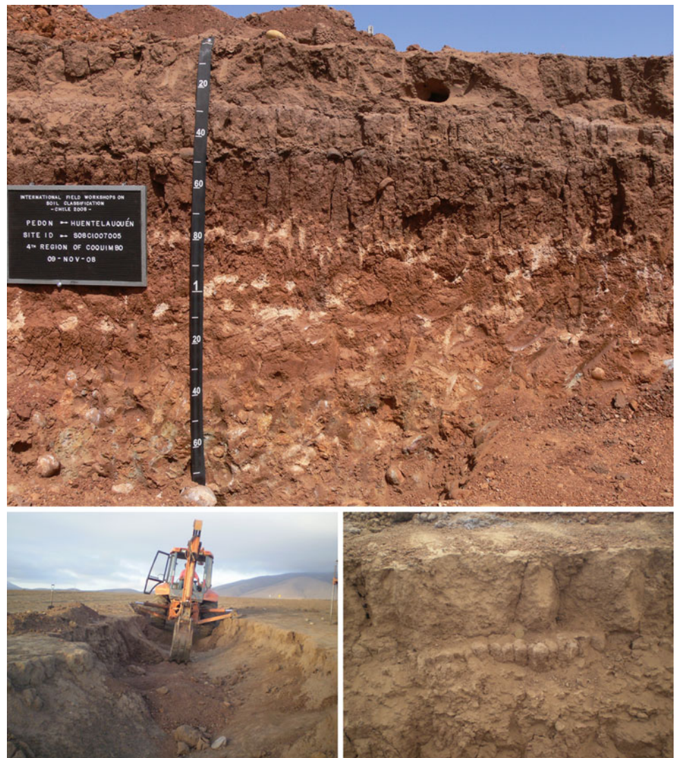
Fig. 2.41 Sodicity features of the Huentelauquén pedon on marine terraces of Region IV
