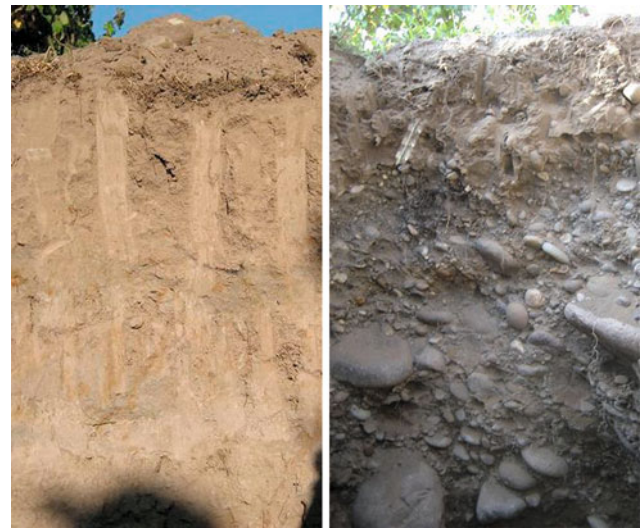
Fig. 3.13 Upper 100 cm in a Fluventic Haploxeroll (left, Isla Huechún soil series) and in an Entic Haploxeroll (right, Codigua soil series), both located in the same alluvial terrace of Mediterranean zone, separated by 20 m. Differences between soils determine a water availability of 16.7 and 6.6 cm, respectively (Ibáñez 2009)
