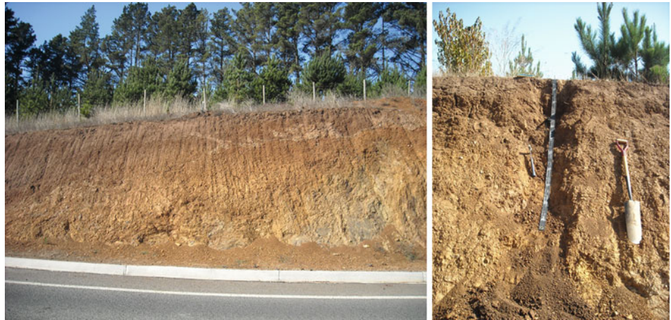
Fig. 2.6 Coastal Range residual igneous soil (Ultic Palexeralf) observed in Regions VII and VIII of Chile
