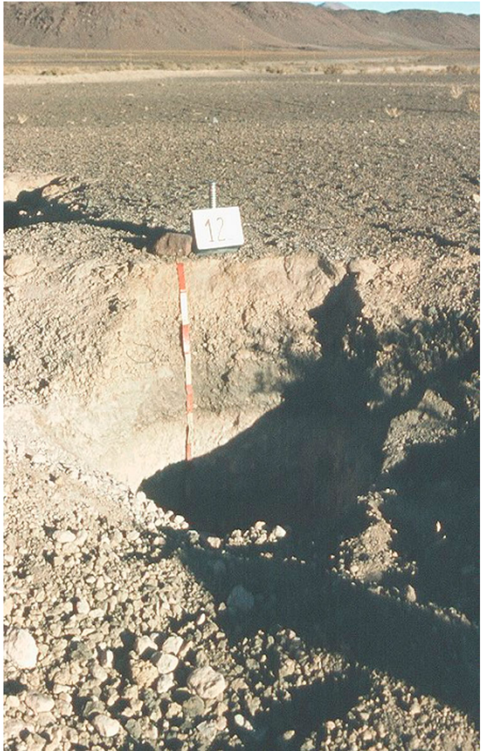
Fig. 2.17 Stratified volcanic soil with abrupt tephra (ashes and lapillis) layers, located between Calama and Ollagüe, Region II (Luzio et al. 2010)
