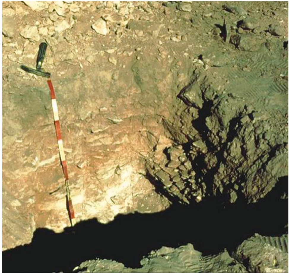
Fig. 2.15 Skeletal soil (Lithic Ustorthent) of 20 cm depth over liparite stone, Region I (Luzio et al. 2010)
