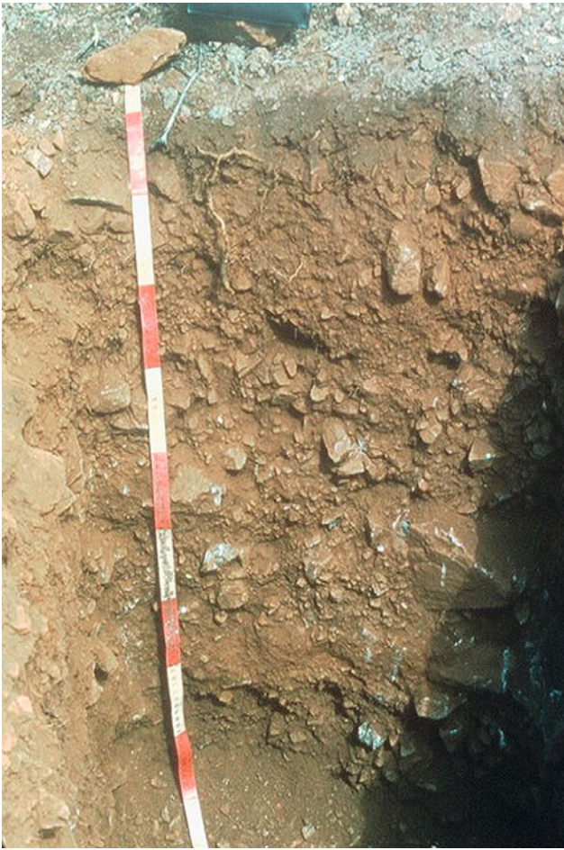
Fig. 2.36 Characteristics of a northern Coastal Range soil profile with colluvial coarse fragments comprising almost 80 % (Luzio et al. 2010)
