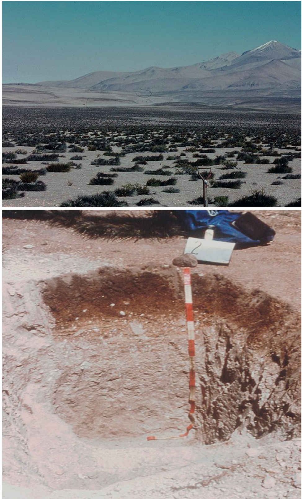
Fig. 2.18 Volcanic origin soil profile ( above ) in sedimentation plain ( below ), located between Putre and Parinacota. Acid pumice ash is apparent in the subsoil, Region XV (Luzio et al. 2010)
