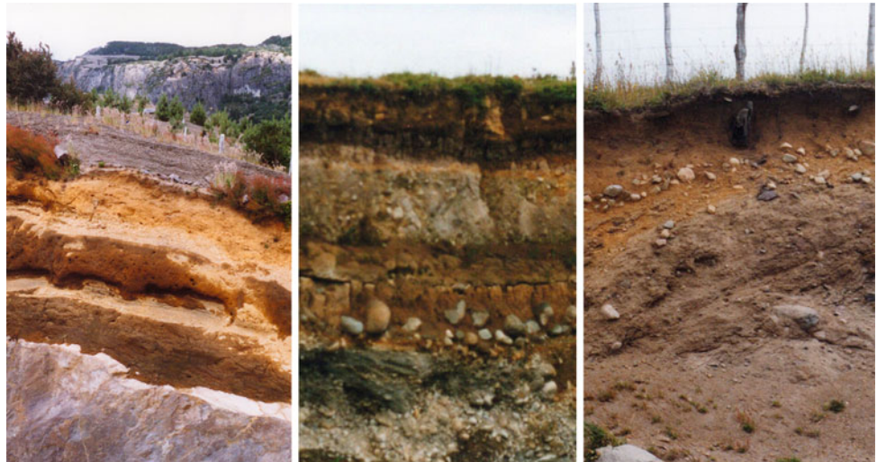
Fig. 2.62 Volcanic soils over different deposits or rocks. Sequence of ash deposited from the Hudson volcano over basaltic rock ( left ), mixed layers in alluvial deposits ( centre ) and volcanic soil over moraine ( right )
