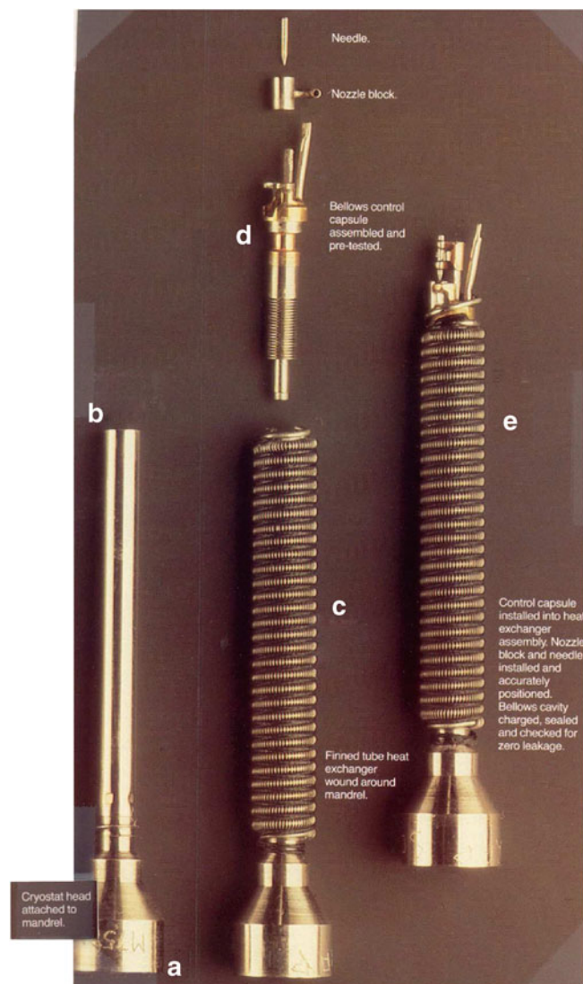
Fig. 6.19 Exploded view of a flow regulated cryocooler of Hymatic Engineering Company, Reddich, England, UK, (a) the inlet nipple, (b) the inner thin mandrel, (c) the finned tube heat exchanger wound on this mandrel, (d) the flow regulating mechanism based on a bellows, including the delicate needle of the valve, and (e) the final assembly
