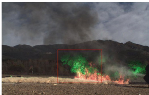
Fig. 2.9 Large-scale particle-image velocimetry of a fire spreading over a vegetal fuel bed in outdoor conditions
