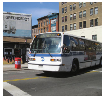
At this intersection, a frequent bus route requires a tight right turn. A recessed stop line paired with a "stop here" sign is used so the bus can complete its turn in one maneuver.
