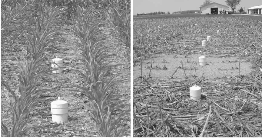
Fig. 17.9 The closed chamber method consists of a gas sampling chamber made of PVC with a bottom section (30 cm long \times 15 cm diameter) inserted into the ground, and a lid equipped with a gas sampling port (Photo by H. Blanco). Air samples withdrawn from the chamber are stored in evacuated vials for the soil gas (e.g., CO 2 , CH 4 ) analyses
