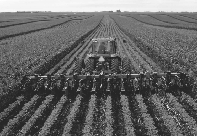
Fig. 8.12 A ridge tillage field used for soil and water conservation (Courtesy USDA-NRCS). Each ridge supports one single row of plants. Tillage and planting are done on the same ridges year to year
