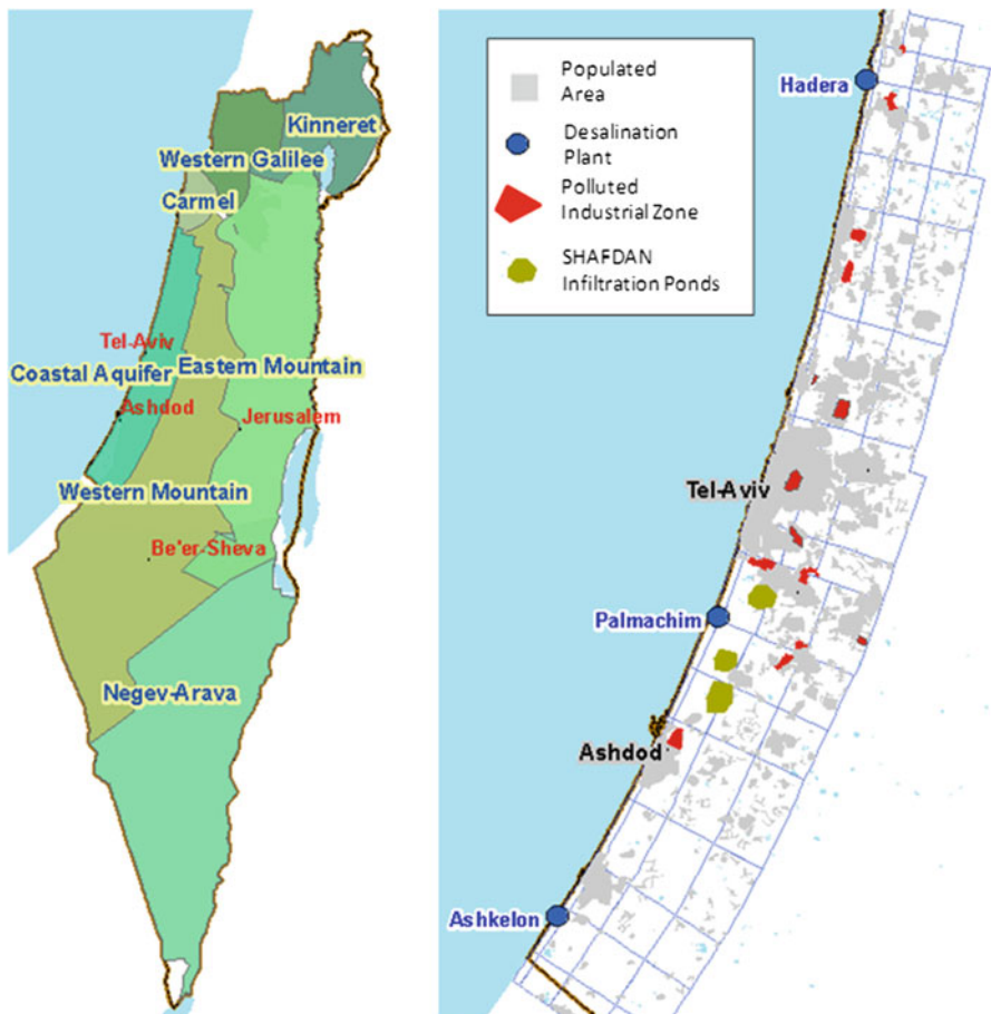
Fig. 8.1 Schematic map of Israel ( left ) presenting major aquifer and surface water systems, major wastewater and desalination plants, and closer map of the ICPA ( right ) indicating desalination plants, the SHAFDAN facility, and populated areas
