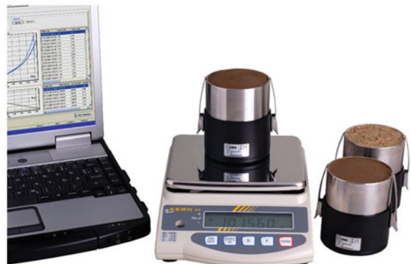
Fig. 6 Sample is clamped, placed on a balance and connected to a computer (photo courtesy of UMS GmbH Munich)
