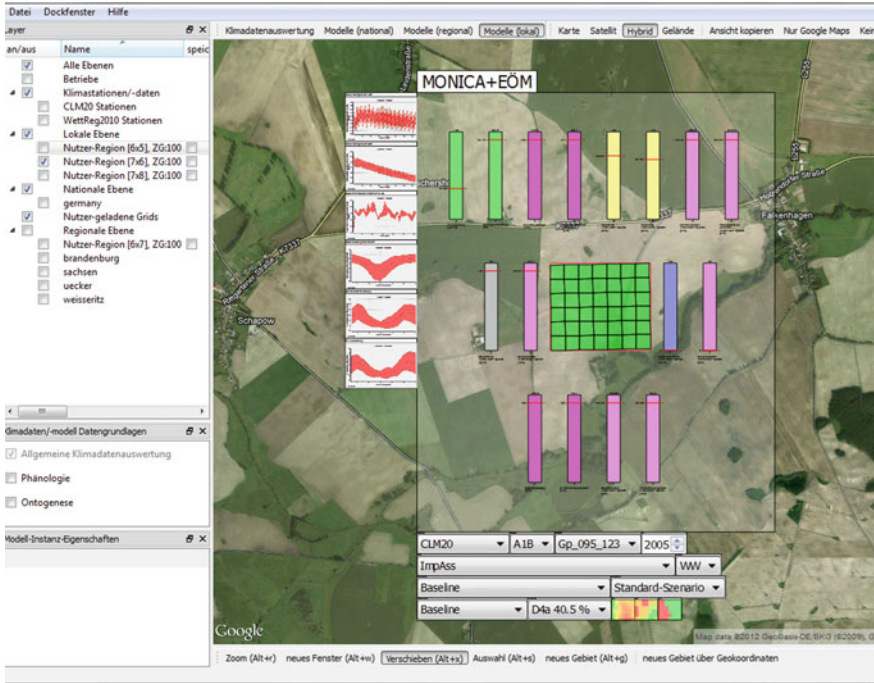
Fig. 5 User interface of the LandCaRe Decision Support System with MONICA plot-scale simulation results displayed in a result panel. Zooming into the panel reveals more details of the simulation results
