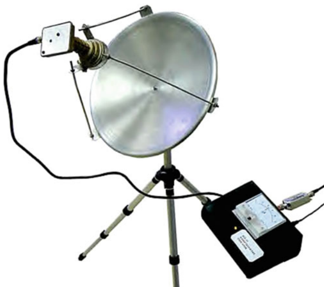
Fig. 11 The RTL-11 Portable Radio Telescope utilizes the same Ku-band receiver as that designed for our purposes, but uses the more directional 32-cm (1-ft) diameter parabolic antenna
