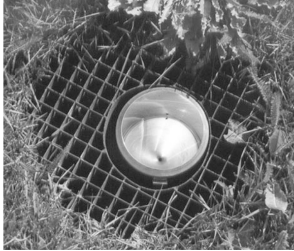
Fig. B.9 Rain gauge with opening at ground level surrounded by an egg-crate structure to prevent in-splashing and errors due to aerodynamic effects (Photo by N. Mölders 2000)
