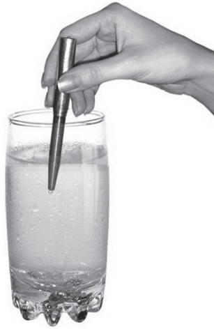
Figure 6. Usage of Pen-Sized Water Disinfection Device.
