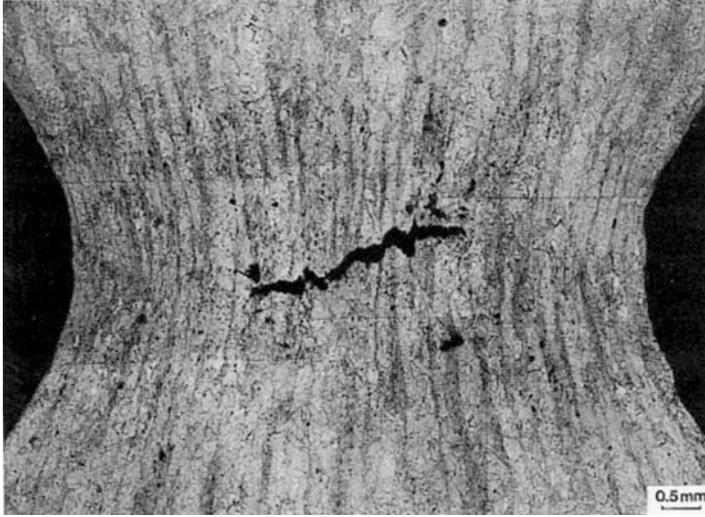
**Fig. 1.58** Longitudinal section through a tensile tested specimen, test of which was interrupted before fracture, showing a crack in the central region of the neck
