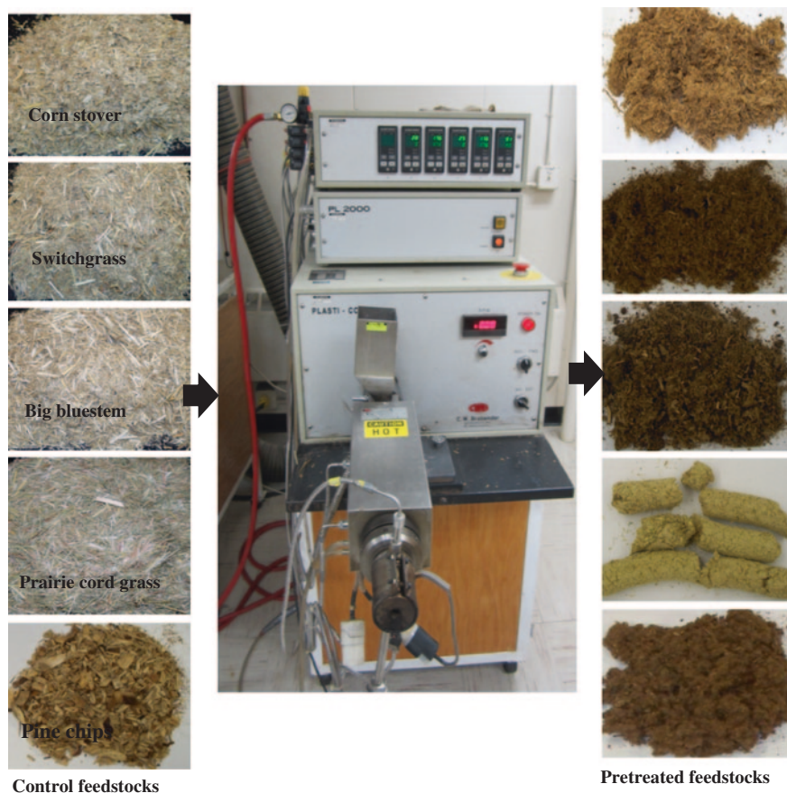
Fig. 2.6 Feedstocks pretreated in a single screw extruder
