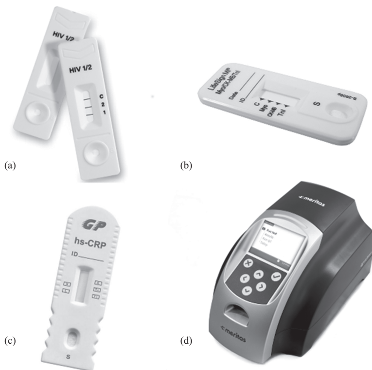
Figure 14.2 Lateral-flow rapid tests and system: (a) an HIV rapid test, (b) a multiplex rapid test for Troponin I, Myoglobin, and Creatine Kinase-MB, (c) a semiquantitative rapid test for CRP-based on reference lines, (d) Meritas by Trinity Biotech: a device-based LFIA with fluorescence detection for quantitative testing of Troponin I and Brain Natriuretic Peptide
