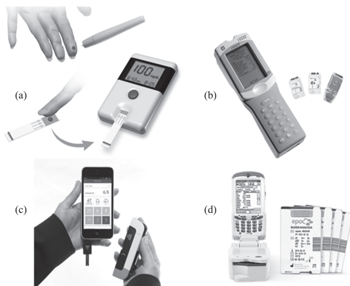
Figure 14.6 Electrochemical biosensing systems: (a) typical glucose meter, (b) i-STAT handheld blood analyzer, Abbott Point of Care Inc. (c) Dario's smartphone compatible glucose meter, and (d) Epoc PoC system by Alere
