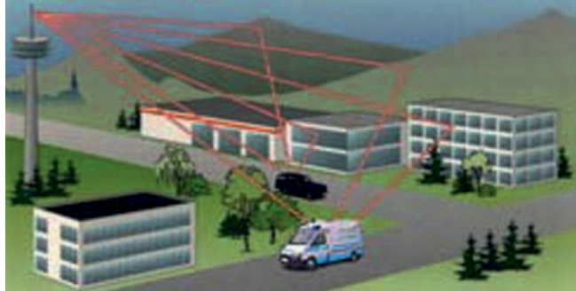
Figure 6. Interference of large structures en route to the hospital
