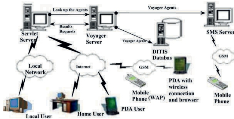
Figure 8. Schematic of DITIS system infrastructure
