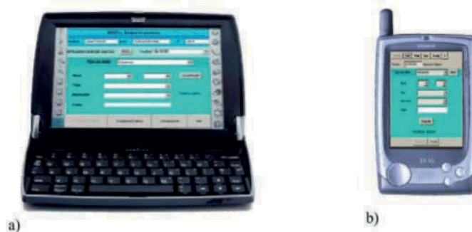
Figure 2: Mobile Patient Units. a) Psion netBook™ (resolution of 640x480 pixels); b) Siemens SX-45 PDA (resolution of 320x240 pixels)
