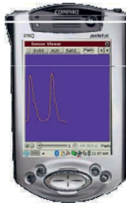
Figure 2. MBU platform (iPAQ H3870), displaying output from pulse oximeter
