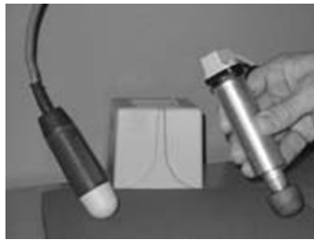
Figure 5. Input device: passive fictive probe designed for the OTELO expert station shown with a 3.5–5MHz ultrasound probe attached to the robotic probe holder system that is located at the patient station
