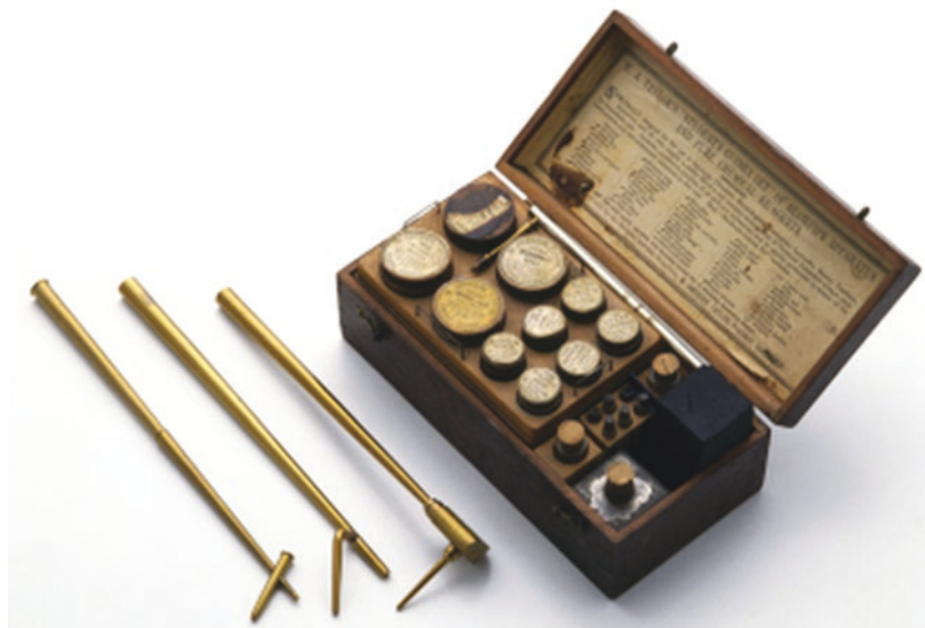
Fig. 1 Blowpipe kit (made by W. A. Taylor of Penzance) and reproductions of three mouth blowpipes which belonged to the English chemists William Hyde Wollaston (1766–1828), Smithson Tennant (1761–1815) and the Swedish chemist Tobern Olaf Bergman (1735–1784), nineteenth-century. Courtesy of the Science Museum/Science & Society Picture Library
