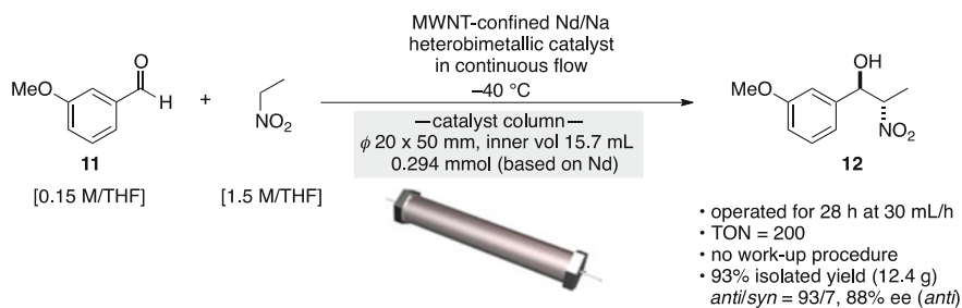
Scheme 8 anti -Selective catalytic asymmetric nitroaldol reaction in a continuous-flow platform
