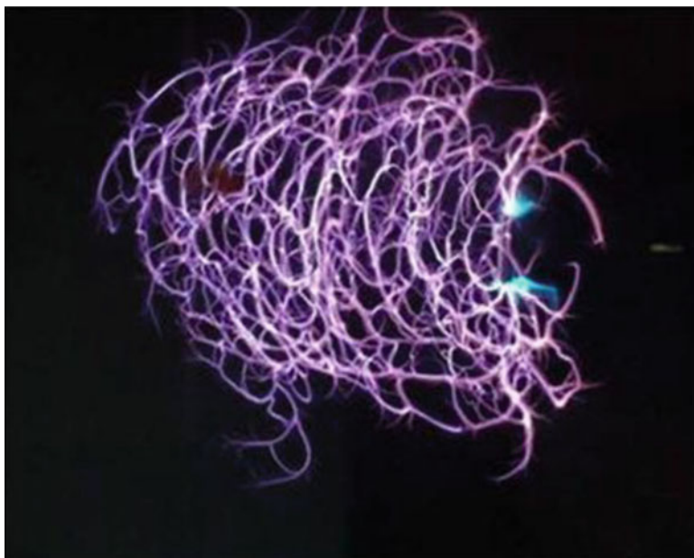
Fig. 5.29 Network of streamer channels in the microwave (MW) streamer subcritical discharge
