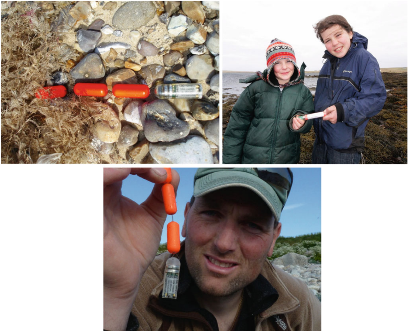
Fig. 1.16 A modern-day message in a bottle, designed to fit into an eel and record details of its spawning migration ( top left ). The recovery of tags depends on the cooperation of an increasingly interested public, as
