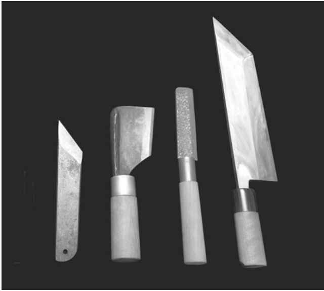
Fig. 6.11 Four representative types of knife used to prepare eels in Japan. From left to right, the Osaka type, a simple pointed blade, the Kyoto type, which is heavy and specially designed for splitting eels, the Nagoya type, a smallish kitchen knife, and the large Kanto (Tokyo) type, used to cut up eels as well as to split them. The Osaka type, originally used for preparing daggertooth pike conger, was probably the prototype, and the Kanto type has become differentiated into the most evolved form and function. Although used for the same basic purpose, these types of knife all remain in use today, reflecting local methods of preparation and the preferences of local eel chefs
