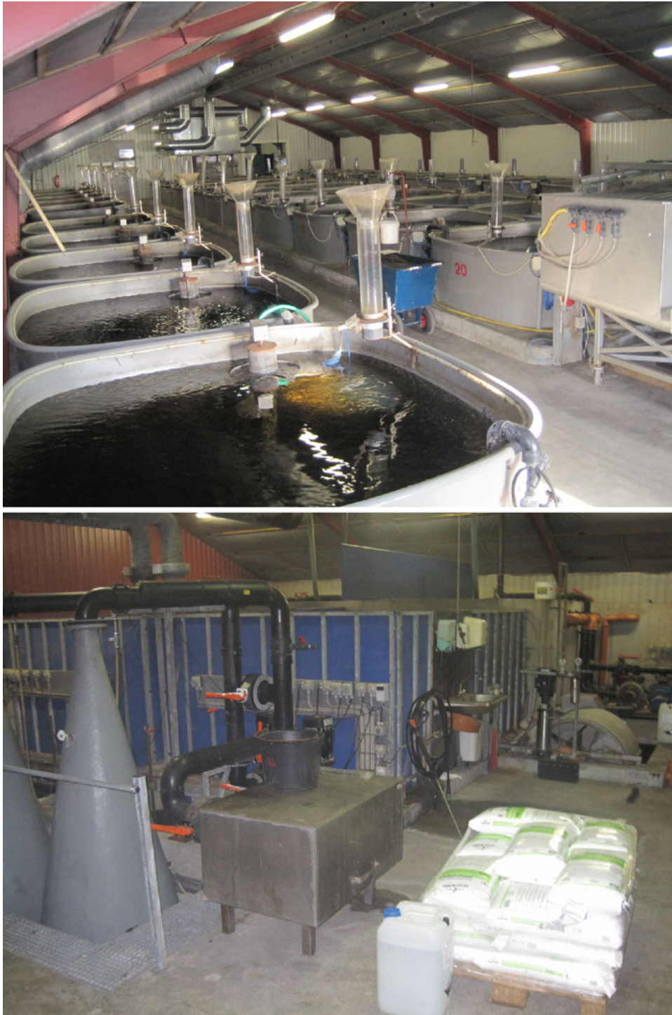
Fig. 3.10 Fish tanks at a Danish eel farm ( top ), and a filter unit with submerged and trickling filters, oxygen cones, pumps, UV-sterilizer, micro-sieve and pumps (photographs, Christian Graver, Danish Eel Farmers Association)
