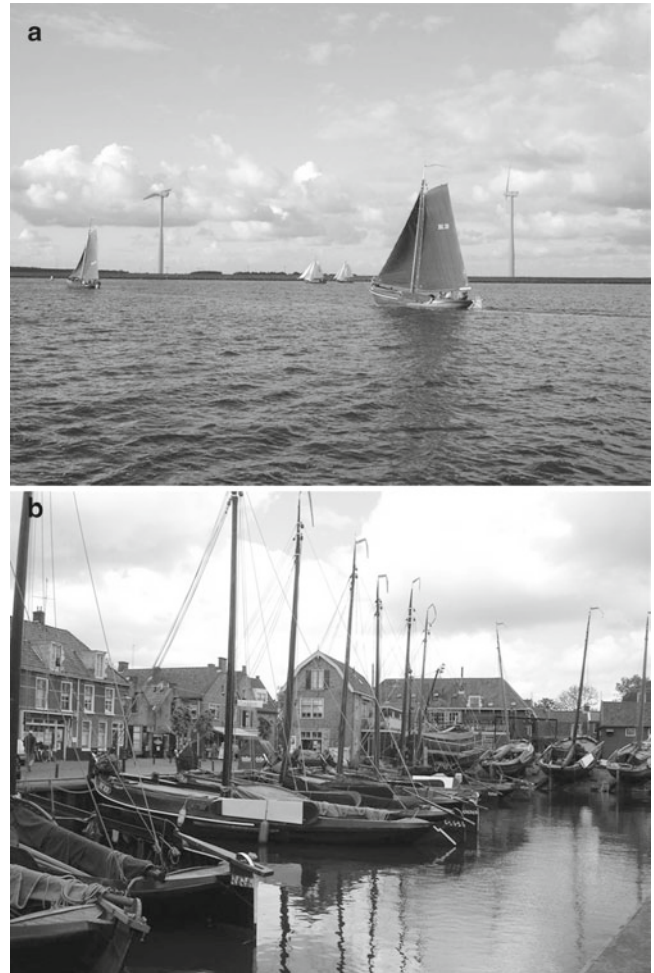
Fig. 4.3 (a) Traditional fishing boats (“Zuiderzee Botters”) still sail on IJssel Lake, but just for recreation. The boats are built for shallow water; they have side boards that are lowered when the winds are from the side to act as a keel. (b) Many of them are berthed in Spakenburg, an old Dutch eel-fishing village
