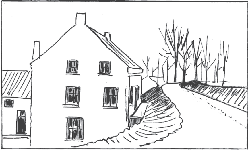
Fig. 9.13 The result of a number of dike-reinforcements at the Waal ring-dyke in Rossum, Bommerlaerwaard. The house was built in the late 18th century. The front door of the house was situated on the crown of the dyke before 1861. After the flood of 1861 the dyke has been raised ca. 1 m; the road is on top of the dyke. After the narrow escape from the flood of 1995 the dykes have been heightened again with ca. 0.7 m, which shows on the right (Drawing P.H. Nienhuis)
