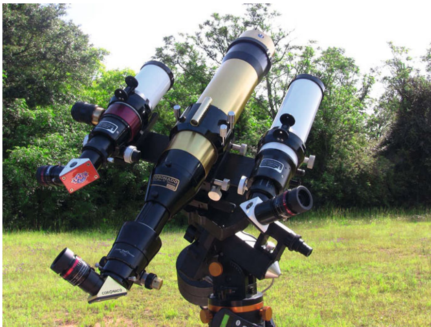
Fig. 6.14 Three solar telescopes in one! The left scope is a Lunt LS60 THa with pressure tuner (on the mid-side). The right scope is a 60 mm Lunt LSTHa with a standard tuning ring. The middle scope is a 90 mm Coronado SolarMax II (Courtesy of Stephen Ramsden).
