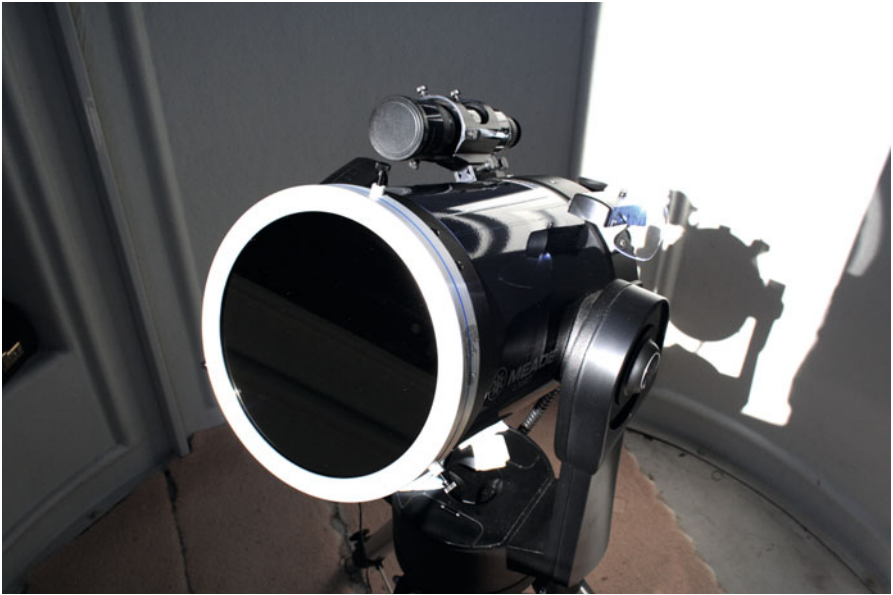
Fig. 6.4 A glass type solar filter mounted on the front of the author's SCT telescope objective lens. Notice that the cap of the finder scope is in place, so the Sun's image does not melt the cross hairs inside and so that you do not look through it. Align the scope using the Sun's shadow of the scope.
