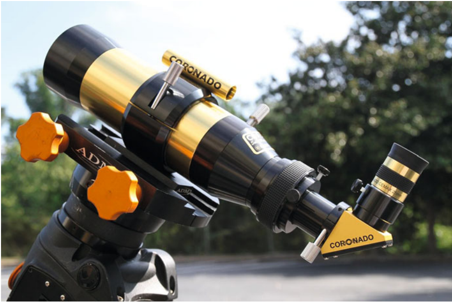
Fig. 6.12 A SolarMax II 60 mm scope being used to view the Sun in H-alpha light (Courtesy of Stephen Ramsen).
