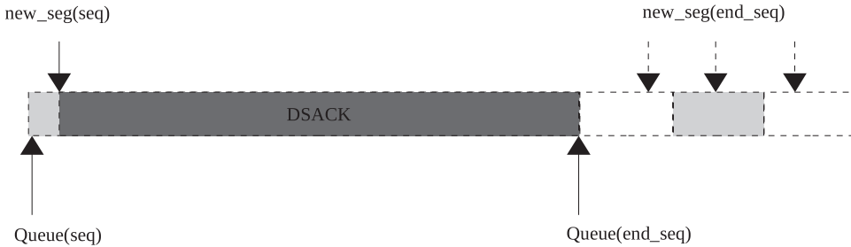
Figure 11.16. DSACK blocks generated in case new out-of-order segment spans across several segments in an out-of-order queue.
