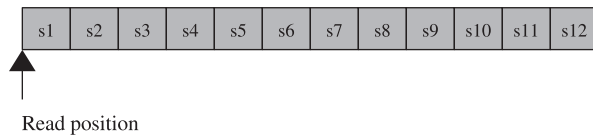
Figure 2.26a. Receive buffer is full.
