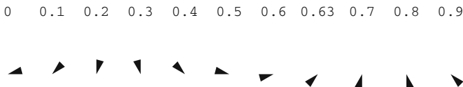
Fig. 13.22 Each sector of circle represents a resonance between two linear oscillating modes \omega_n and \omega_m ( n < m ) for a three-dimensional inviscid drop with rigid core. \epsilon is the radii ratio core/drop. While the core extends (in the figure the black sector rotates CCW) some resonances vanish, some new occur, and some are stable
