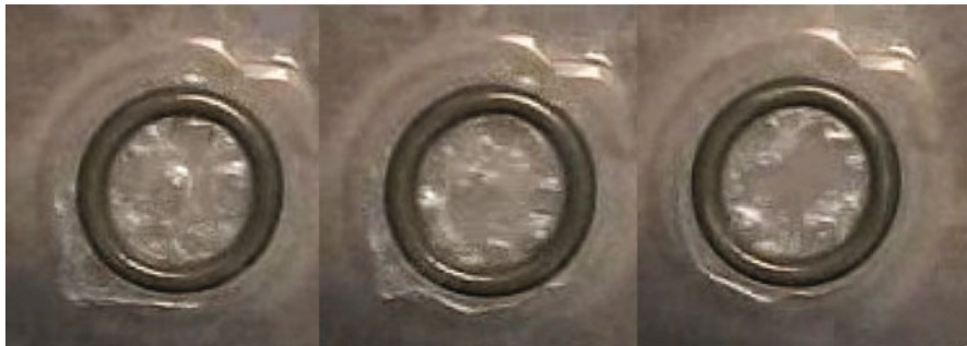
Fig. 12.14 Traveling and decaying of cnoidal waves on the external contour taken at three different moments of time
