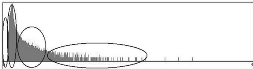
Fig. 10.3 The typical histogram for astronomical images has four major areas of interest, as shown here
