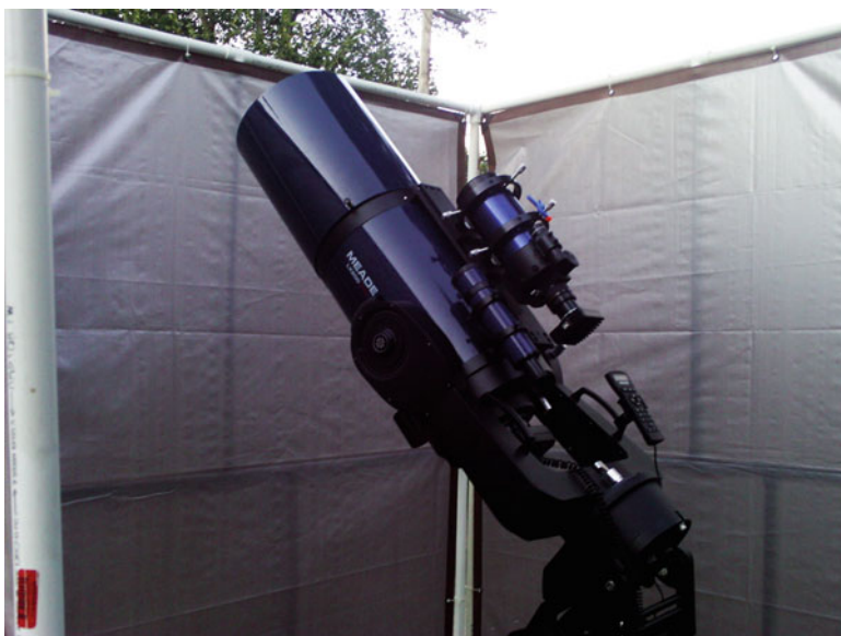
Fig. 2.6 A windscreen can be used to prevent the wind from causing any vibrations of your telescope, which are magnified greatly onto your images
