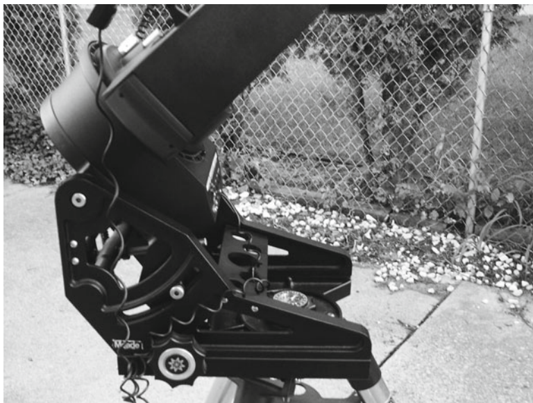
Fig. 2.3 A wedge platform that helps you get your telescope into polar alignment
