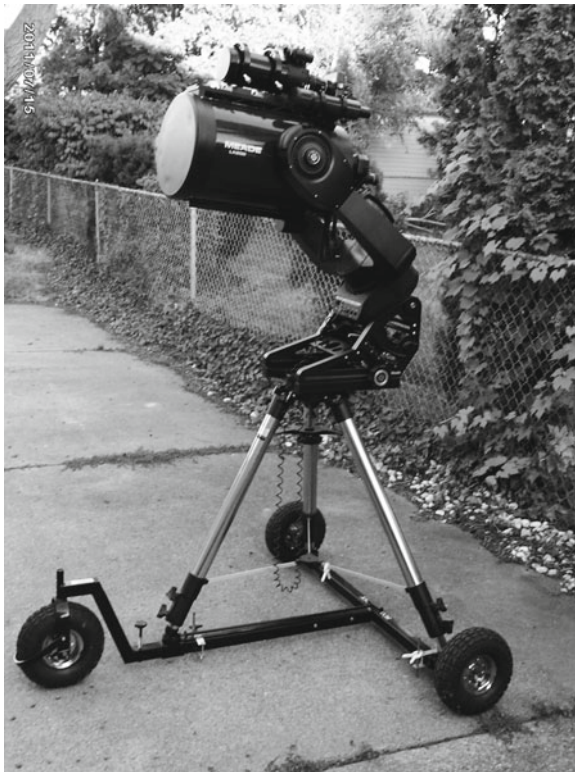
Fig. 2.4 An SCT telescope with a wedge platform sitting on a three-wheeled 'scope cart
