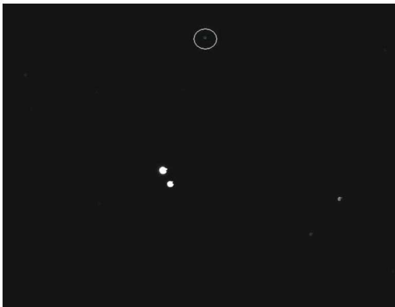
Fig. 6.11 With the brighter stars focused, fainter stars will start to appear; use these smaller stars to fine-tune your focusing
