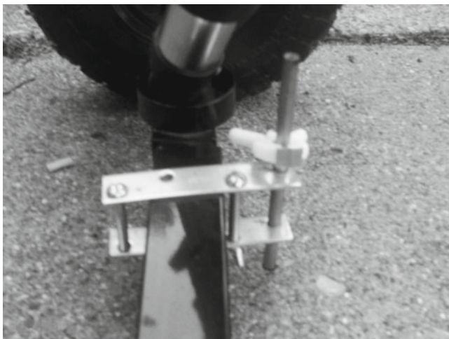
Fig. 5.1 A dropdown rod attachment for your 'scope cart provides exact precision in setting up your equipment for each imaging session
