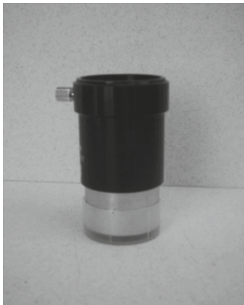
Fig. 4.10 A Barlow lens is used to decrease the field of view for a given telescope/imager combination
