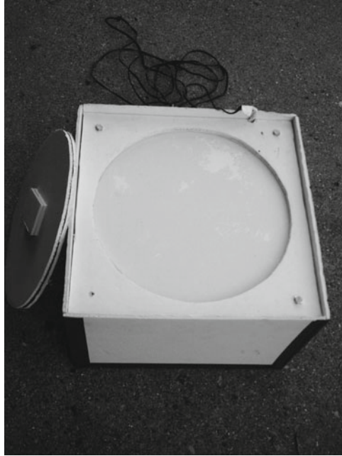
Fig. 7.8 A light box enables you to take flat-field images immediately following the imaging of a specific target so you can make configuration changes when you move onto the next target
