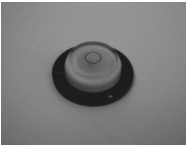
Fig. 2.7 A bubble level is used to level your telescope's base during setup
