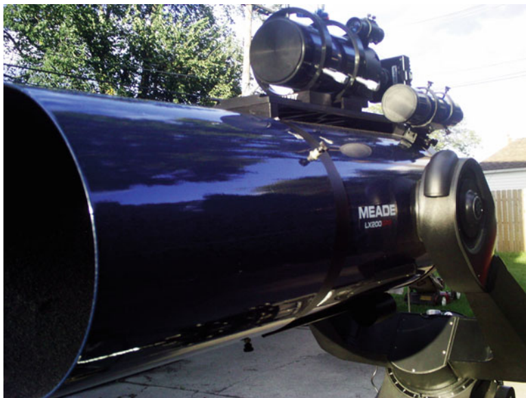
Fig. 8.4 A smaller telescope can be piggybacked onto your larger telescope along with another CCD camera for use in auto-guiding
