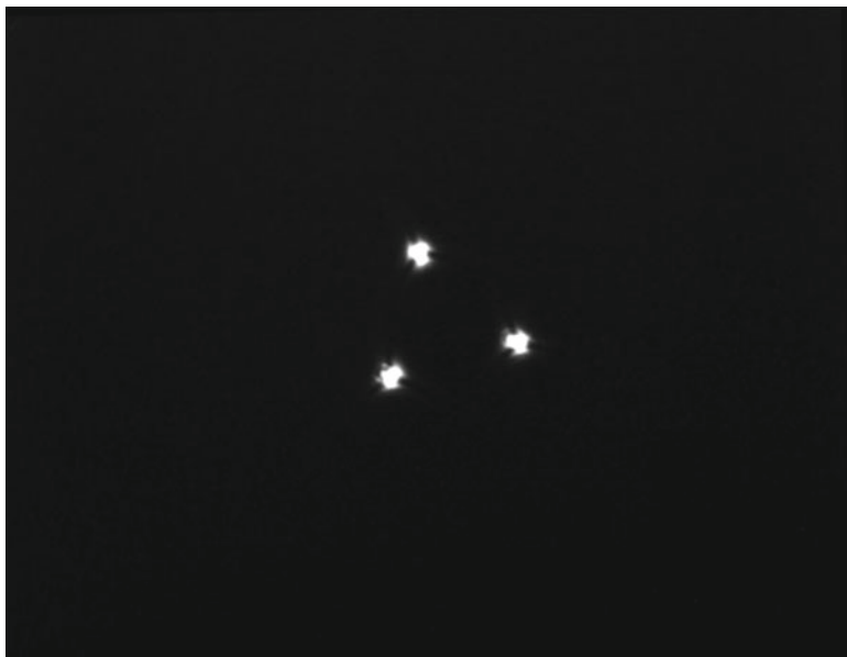
Fig. 6.2 With a Hartmann mask in place, three shapes appear on your imaging program's display
