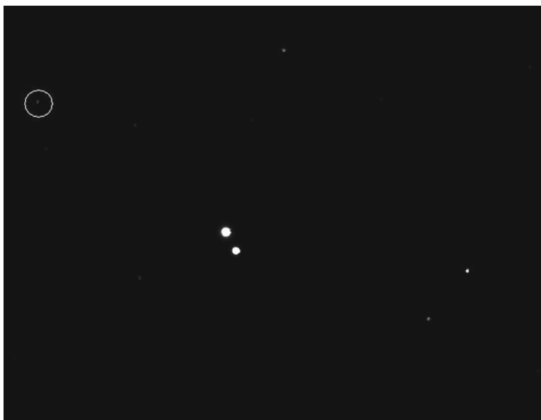
Fig. 6.12 As you get closer to the critical focus zone, you will start to see more and more, even fainter, stars in your imaging display
