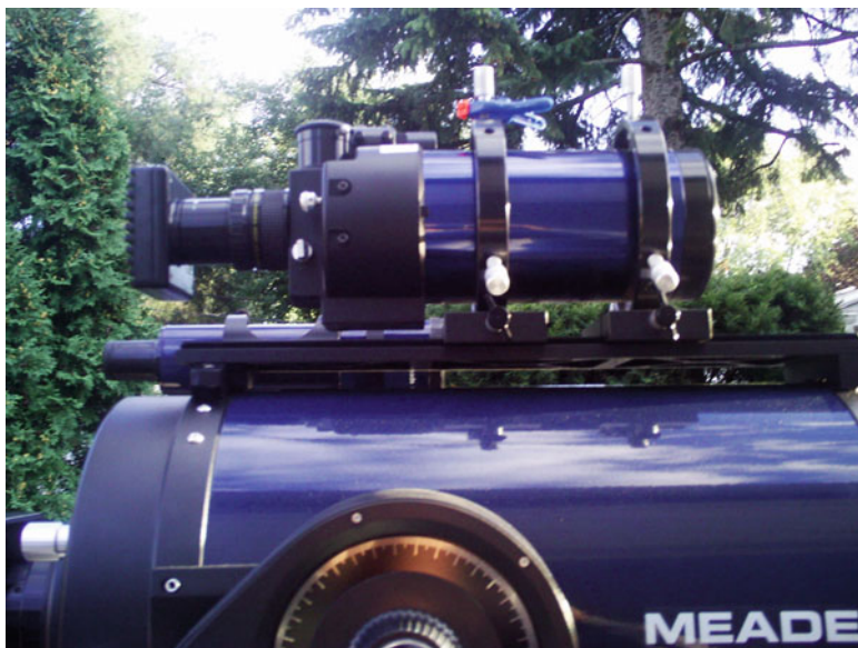
Fig. 3.2 An auto-guiding telescope and CCD camera “piggybacked” onto the main telescope will be used to keep your imaging subject on the same pixels of the imaging chip
