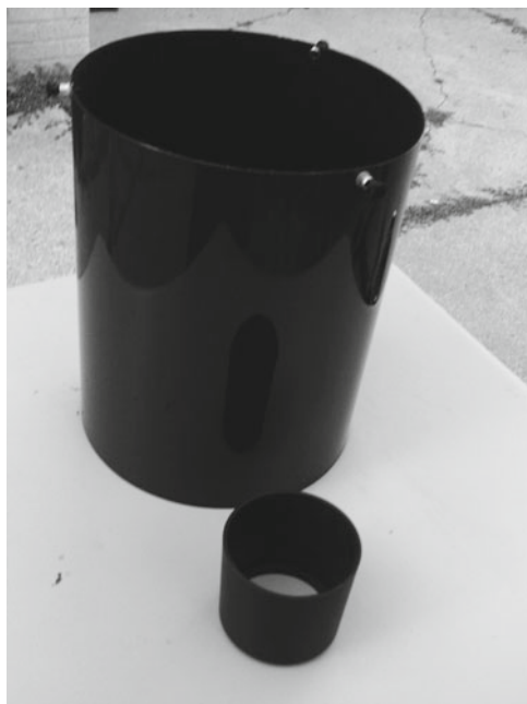
Fig. 2.8 A dew shield extension for your telescope will help prevent the onset of condensation on the lens
