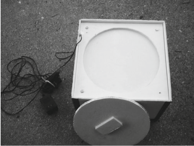
Fig. 2.11 A custom-made light box used for image calibration (Courtesy www.digitalspaceimages.com )
