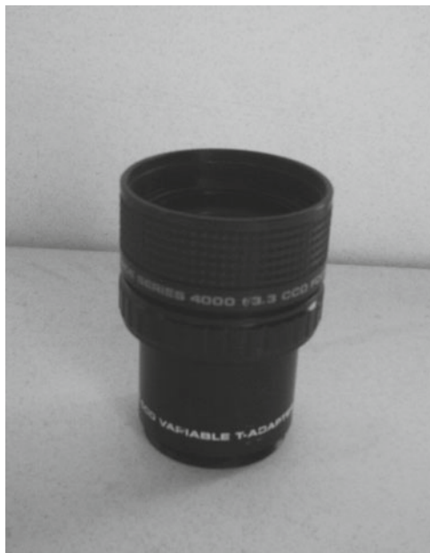
Fig. 4.9 A focal reducer is used to increase the field of view for a given telescope/imager combination
