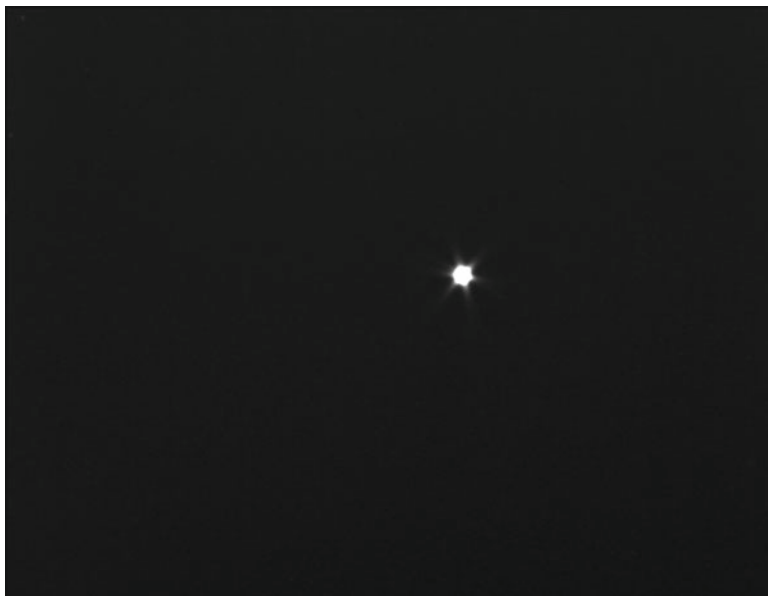
Fig. 6.7 Your rough focus is finished when the star is crisp and the diffraction spikes from your mask are as long as you can get them
