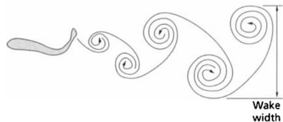
Fig. 5.32 Typical wake behind a swimming fish.
