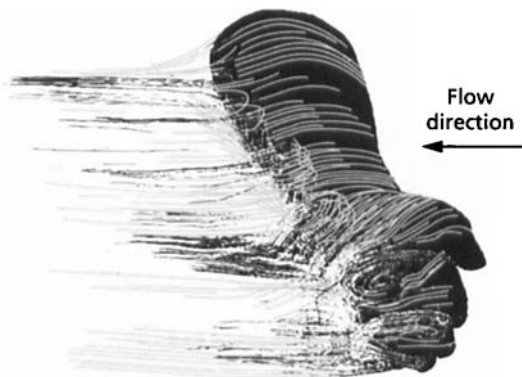
Fig. 5.10 Flow path lines around a swimmer's hand and arm show significant boundary layer separation.
