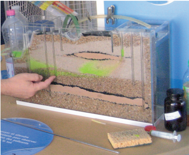
Fig. 8.5 Photograph of a vertical slab physical model of groundwater flow in a heterogeneous aquifer system. This scale model was made for qualitative demonstration of flow paths and contaminant dispersion. It was designed in 2006 at the Institut de Mécanique des Fluides de Toulouse (R. Ababou, D. Bailly, E. Milnes, M. Marcoux, et al., Porous Media Group, IMFT, Toulouse, France) in collaboration with J. Langot at Science Animation (Centre de Culture Scientifique, Technique et Industrielle de Midi-Pyrénées, Toulouse, France)
